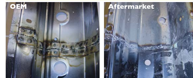
A proper crash part uses backing plates to add strength, mounting points that match the original part, and appropriate bolt-hole sizes and position.
