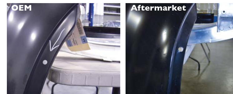
Compared to an OEM part, and aftermarket part can vary in metal type, thickness, and finish, plus the latter's collision characteristics are unknown.
