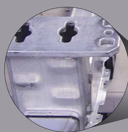
OEM bumper reinforcement: Notice the metal thickness and solid base.
